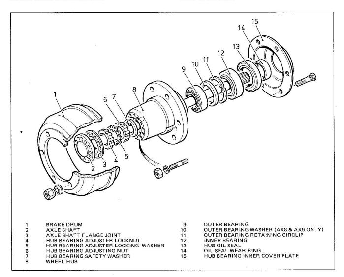
Fig. 3 Hub Assembly General Arrangement
