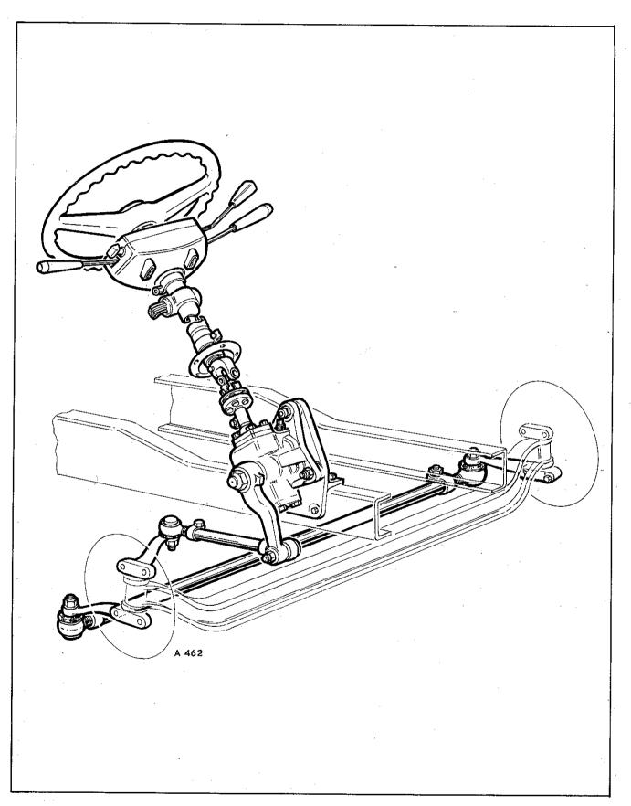
Fig. 1 Layout of steering gear
